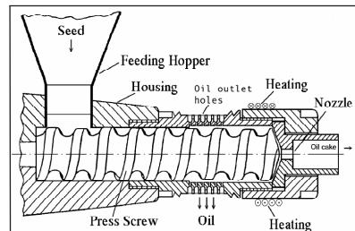
**Figure 1.** Hole cylinder press of a KOMET oil expeller (Ferchau, 2000)
