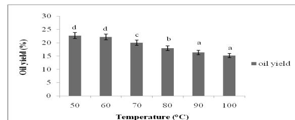
**Figure 2.** Means of percentage oil yield from *N. sativa* seed pressed at six different temperatures. Means in the column with different letters are significantly different ( $p<0.05$ )  $N=3$
